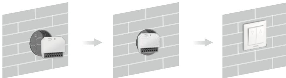
European Installation Method 80 x 80 (mm)
